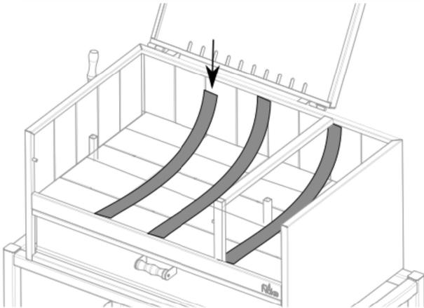
**2** Remove the bricks protectors pulling down to release from the grill body.
