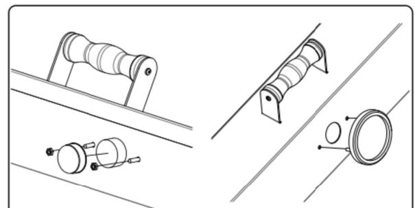
**i** For thermometer replacing, first remove the Thermometer case, then unscrew the nuts. Now you will be able to replace the thermometer.
