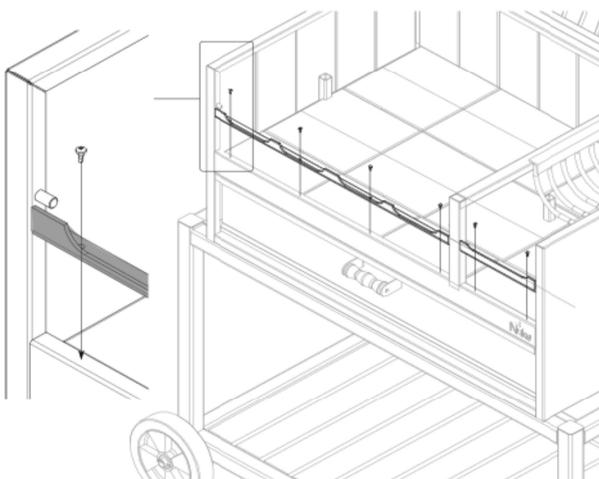
**3** Fix the ember protector to the grill with the self tapping screws. Drilling on grill body.
