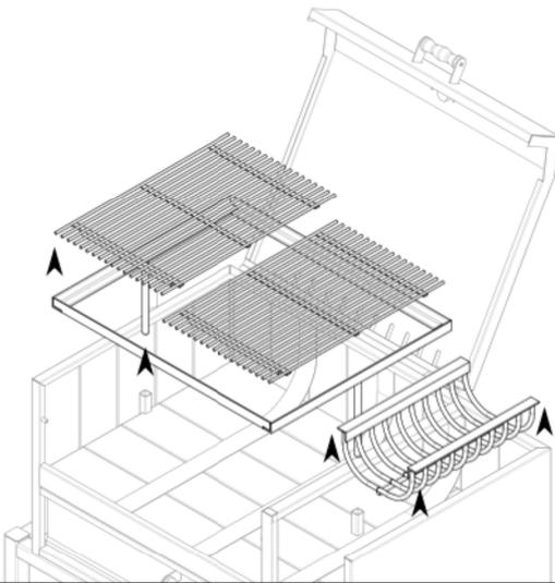
**1** Remove Frame, fire box and grills to continue with DELTA assembly. The parts are not weld so, you just pull up to remove it.
