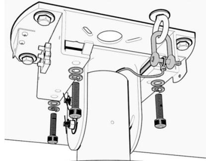
Lift the fan assembly and place it within the ceiling bracket. Secure fan using the bolts and washers provided. **Secure the safety cable into the eye bolt with the shackle. Ensure the safety cable has a slack of 12" to 16".**
