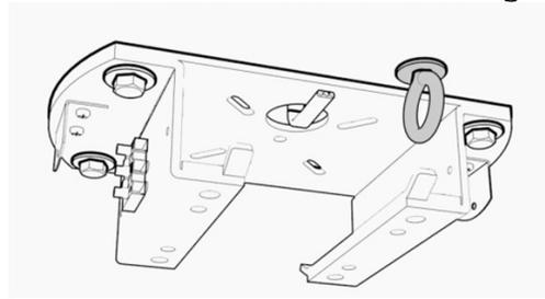
Mount the ceiling bracket using (4) 3/8" or equivalent lag screws . Install the closed eye bolt for safety cable. Ensure eye screw can be covered by the canopy cover.
