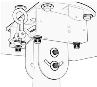
Adjust the hanger tube to be perpendicular to the
