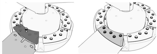
Push the fan blade towards the motor and secure the fan blade using the upper fan blade mount and the 5 bolts. Repeat this with the remaining fan blades.
