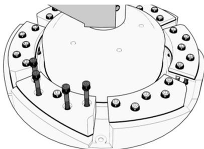
Unsecure the upper fan blade mount by removing the 4 bolts. Loosen the middle bolt.
