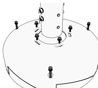
Remove the 5 inner screws followed by the 3 outer bolts
