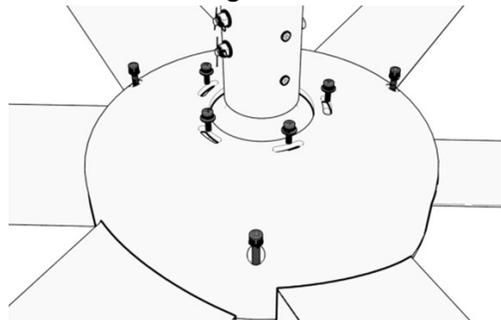
To secure the motor cover, insert and tighten the 3
