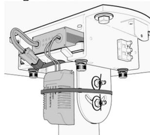
Insert the motor controller box into the fan mount.
