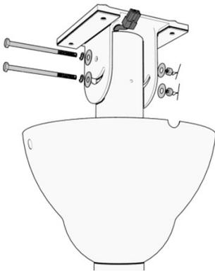
Ensure the canopy cover is inserted into the hanger tube before assembling the mounting bracket to the hanger tube.
