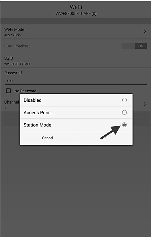
6) Change the Wi-Fi type from Access Point to Station Mode.
